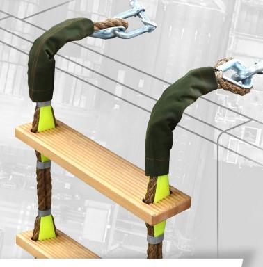
One of the most common reasons for breaking the pilot ladder is its rubbing against the ship's side. To prevent this, use a rubber or wooden edge guard. Secure the top section of the ladder with additional protective sleeves. And check the technical condition of the rope and sleeves each time.
